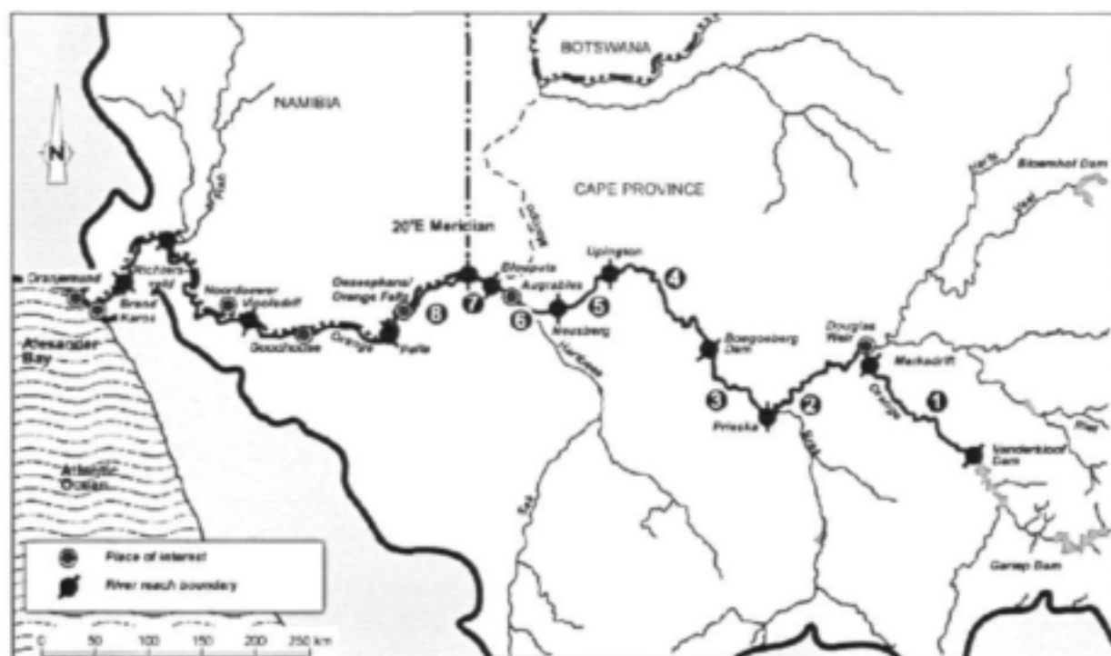
Figure 2-1. General locality map of the middle and lower Orange River, showing tributaries, main towns and eight zones used for hydraulic modelling.
