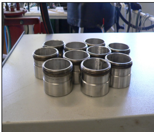
Figure 4-1 : Metal flasks where test dye solution was poured
