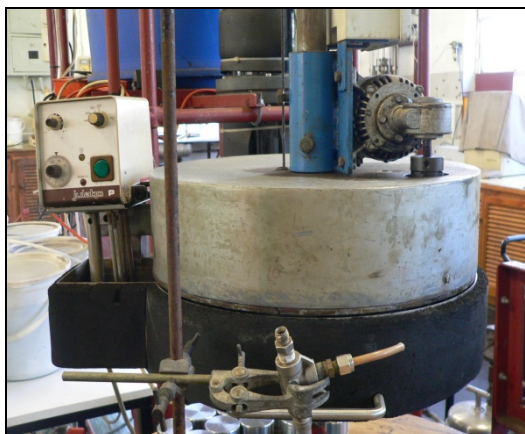
Figure 4-2 : Front view of the stirrers with a temperature controller used
