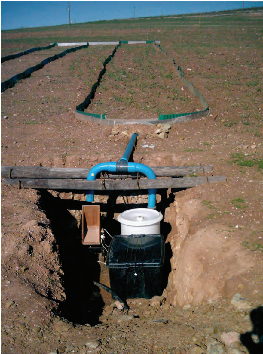
FIGURE 3: Flow splitter, tipping bucket for measurement of overland flow and two plastic tanks for water and sediment sampling
