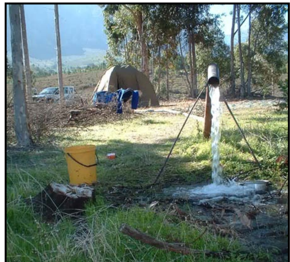
Impacts resulting from pumping tests remain insignificant if the footprint of the camp is kept small and discharge is controlled.
