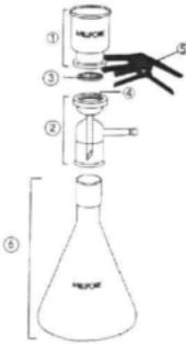
Figure 1. Glass filtration setup (from http://www.millipore.com/catalogue.nsf/docs/C170).
