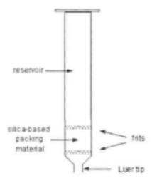
Figure 2. A solid-phase extraction column (from http://www.aquaculture.ugent be ATA code lip\_extr htm).
