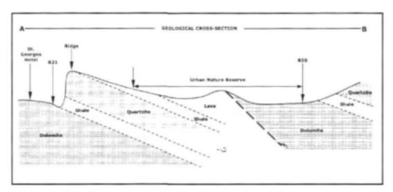
Fig. 3.2: Geological cross-section of Dam 2 area (CSIR communication).
