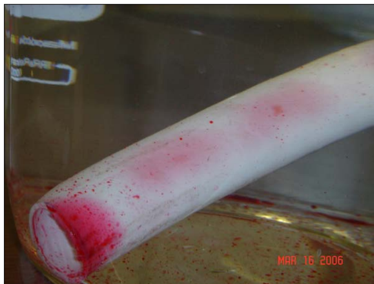
Figure 8: Effect of TCE (dyed red) on PVC material after 11 months of exposure.
