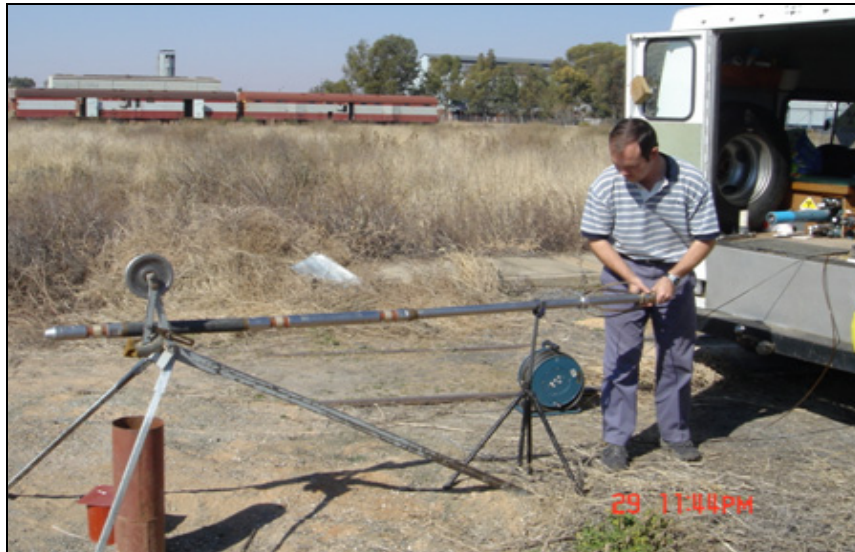
Figure 2: Geophysical logging of boreholes at research site - Test Site 1.
