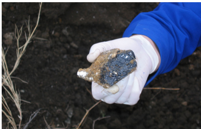
Figure 9: Coal tar visible on soil sample from test pit.
