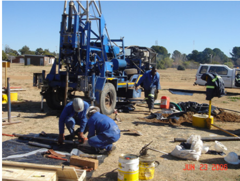
Figure 5: Diamond drilling at UFS Campus Research Site. Note the temporary sump used for circulation of drill fluids.
