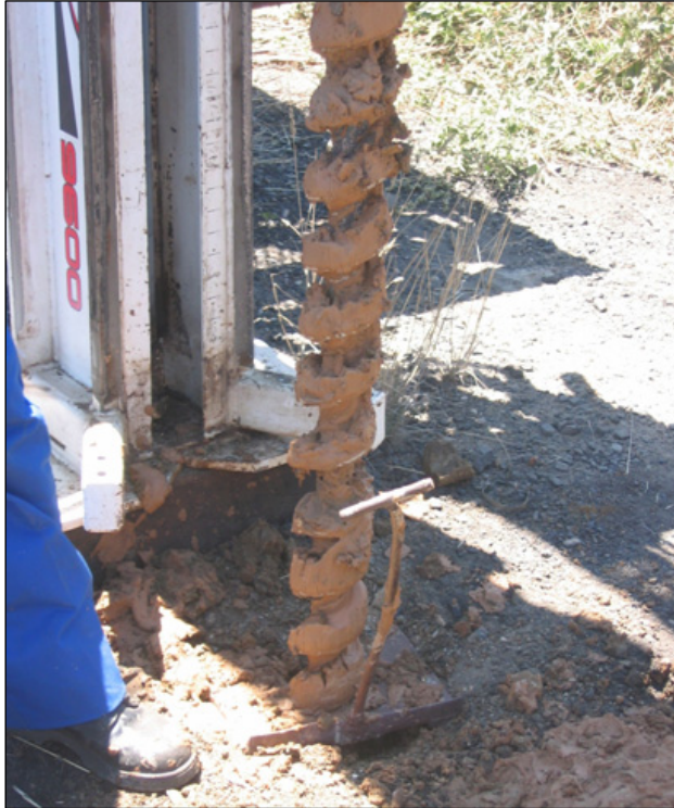
Figure 4: Caking of sand and clay slurry during auger drilling.
