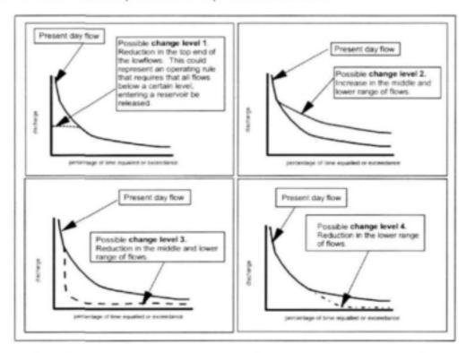
Figure 3.5 Schematic representation of possible alterations to a lowflow FDC, each of which would represent one change level, with an accompanying annual volume and daily distribution.
