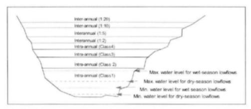
Figure 3.3 An hypothetical example of the water depths delineated by the various hydrological statistics, shown on a cross-section of river channel.
