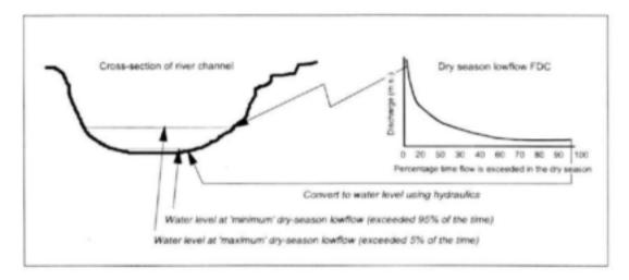
Figure 3.2 The range of hypothetical lowflow discharges that occur during a dry season, expressed as water depths shown on one or more cross-sections of the river channel at each EFR site. The amount of time that the water level was at or above a particular level may be derived from the FDC.
