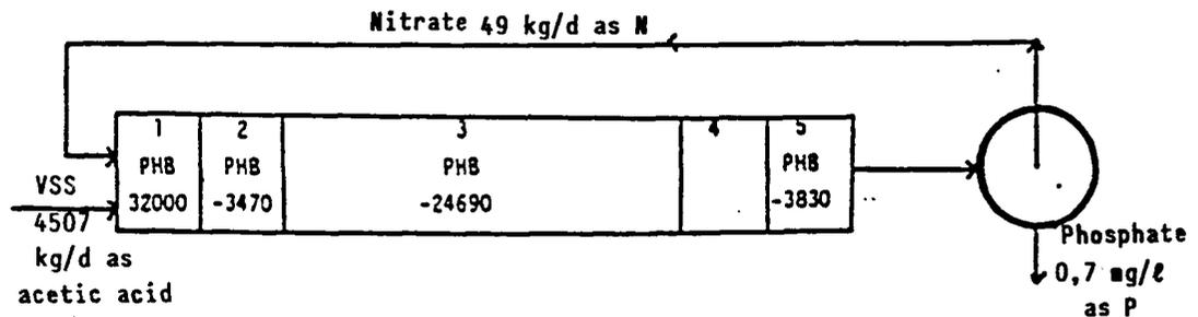
Figure 4.11 : Typical results of PHB synthesis and degradation in Goudkoppies activated sludge plant
