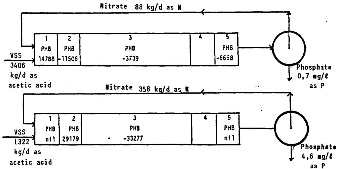
Figure 4.12 : Typical results of PHB synthesis and degradation in Northern Works, Module 2, activated sludge plant - indicates degradation. Results in kg/d
