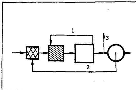
Figure 2.1 : A schematic representation of the three-phase Bardenpho process
