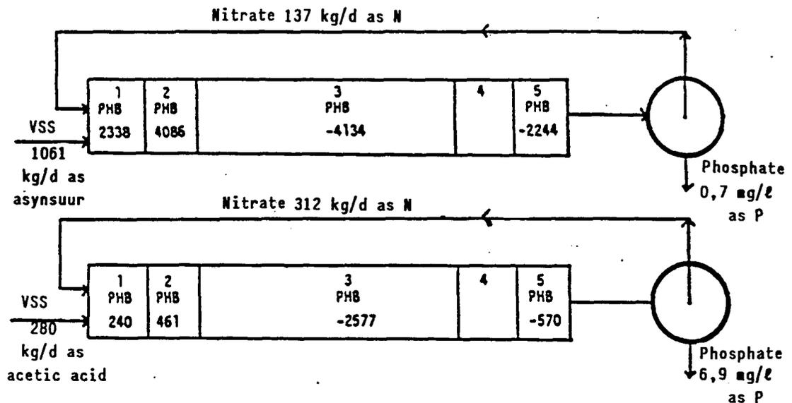
Figure 4.13 : Typical results of PHB synthesis and degradation in Northern Works, Module 3, activated sludge plant - indicates degradation. Results in kg/d
