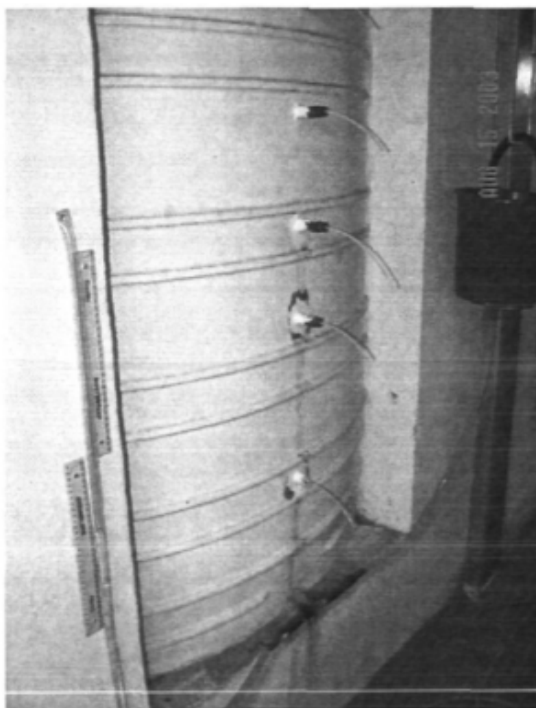
Plate 5.1 Ceramic cups installed from the access chamber side of the lysimeters at different depths from the soil surface.
