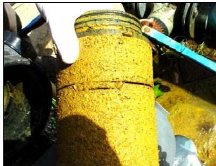
**Fig. 4.1: Dirt build-up on discs and foreign objects between discs at site 5.2**
