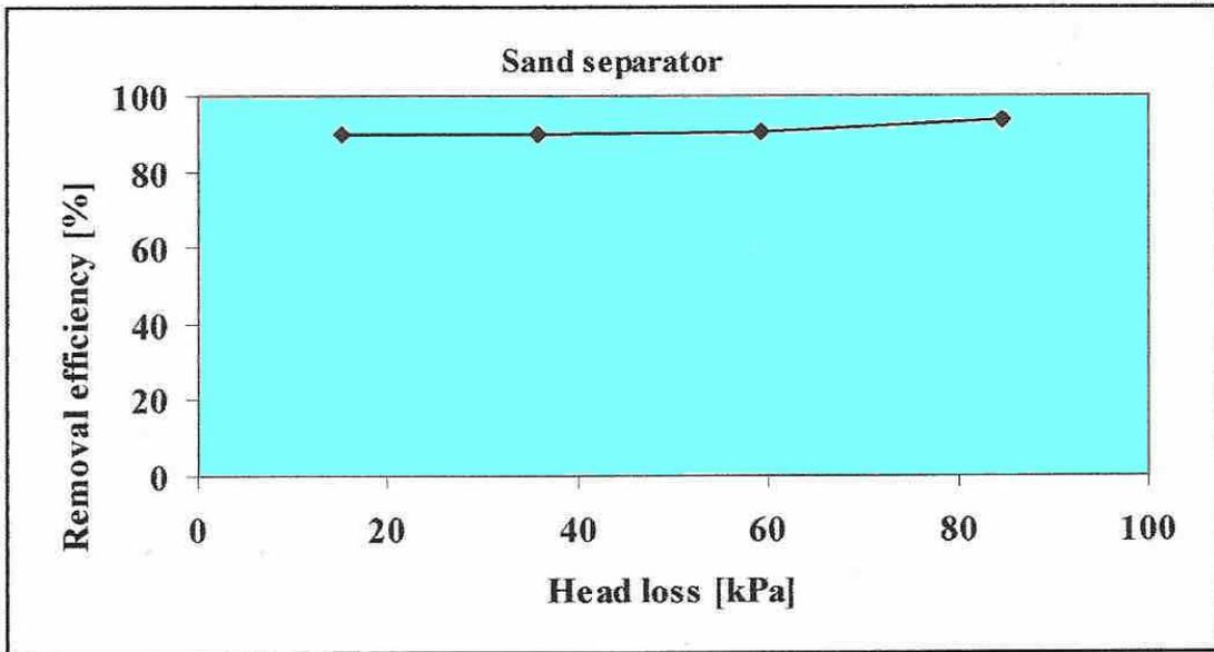
Fig. 2.7: Removal efficiency of a sand separator (after Norum, 1999)
