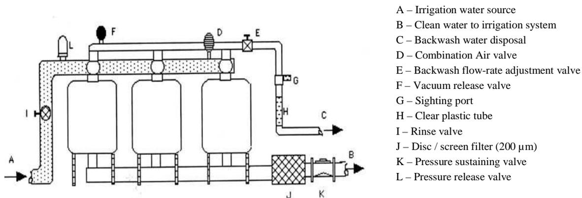
**Fig. 6.1: Typical layout of three sand filters with accessories
