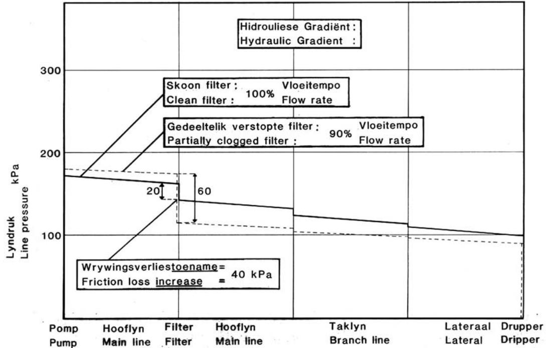
**Diagram 6.1: Permissible friction loss increase over a filter**
