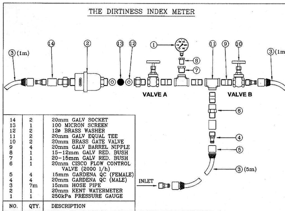
Fig. 1: Construction of the Dirtiness Index Meter
