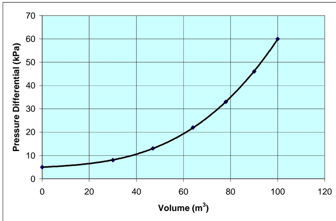
Fig. 2.5: Typical clogging graph of a filter (Van Niekerk, 1983)
