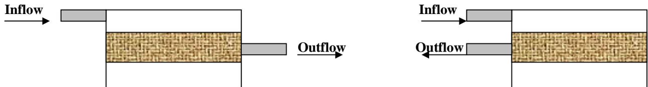
**Diag. 4.1: Different ways of water flow through filters**
