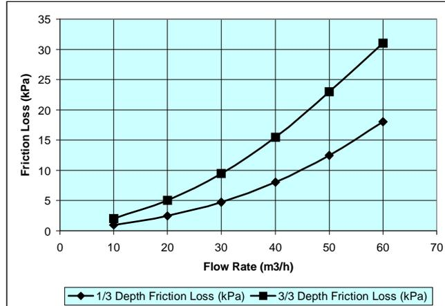
**Fig. 4.14: The effect of the sand depth in a sand filter on its friction loss**
