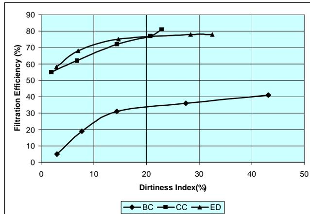
**Fig. 4.15: Filtration efficiency test results on the automatic filters**
