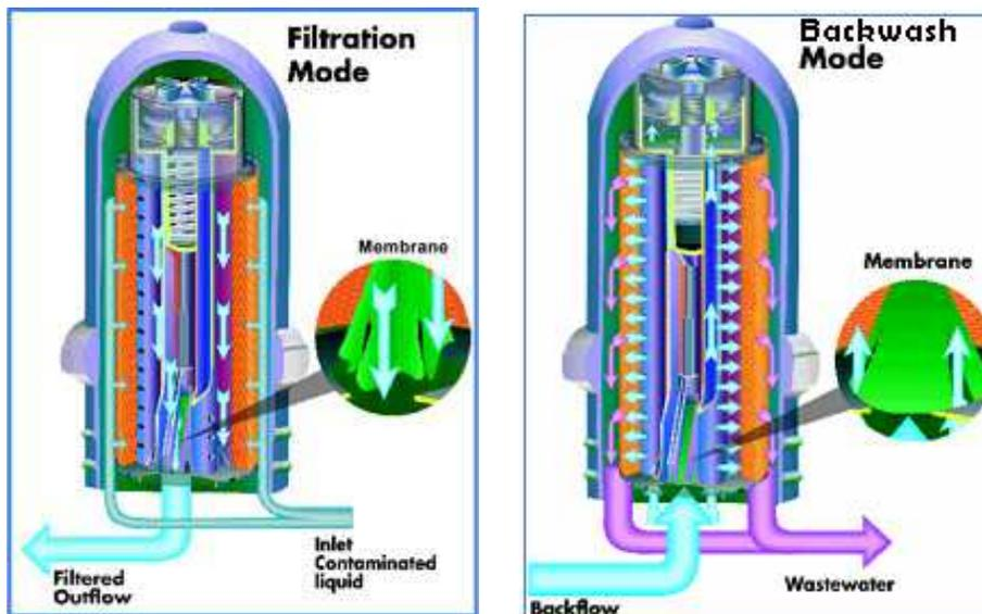
Fig. 2.2: Operating principles of automatic disc filters during the filtration and backwashing mode (Arkal, 2002)
