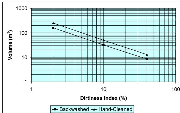
**Fig. 3.3: A typical filtration capacity curve of a filter**
