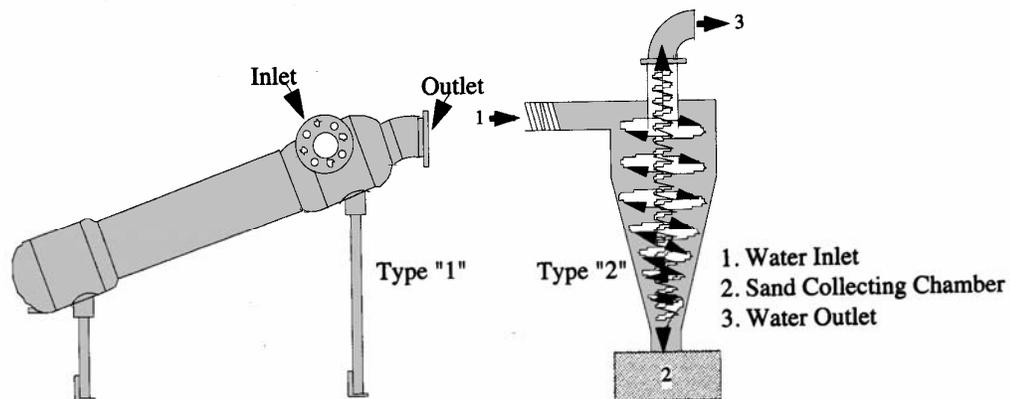
**Diag. 2.4: Two types of sand separators (Burt and Styles, 1994)**
