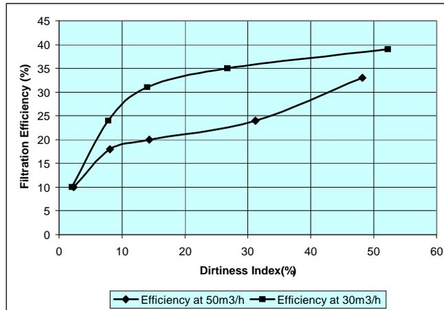
**Fig. 4.17: The effect of flow-rate on filtration efficiency**
