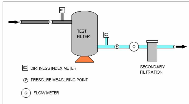
**Diag. 3.2: Schematic set-up of filter test**
