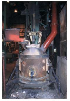
Figure 5.8: The 200 kW DC furnace
