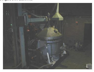
Figure 5.10: 500 kW furnace
