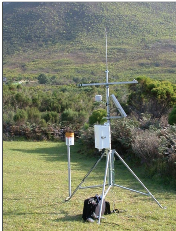
Figure 2-1 The Campbell automatic weather station with relative humidity probes, temperature, wind speed and rain gauge.
