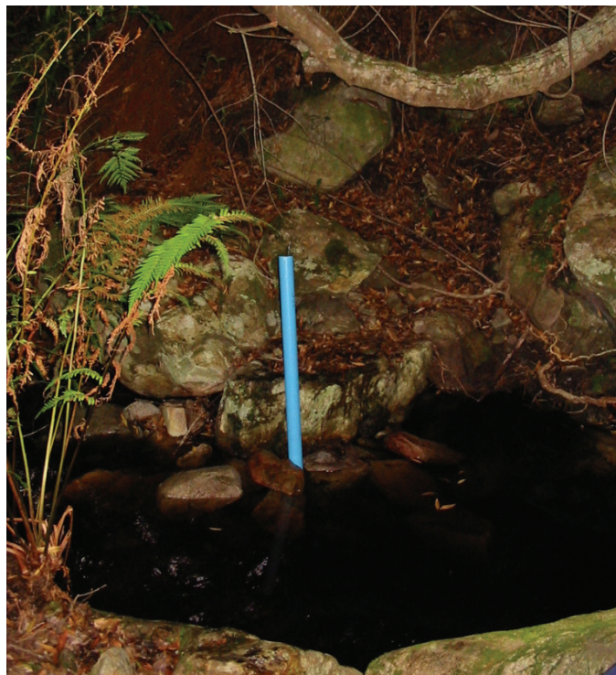
Figure 2-3 L-shaped piezometer installed in a permanent pool in the Oudebos tributary at Kogelberg to house an automated water level data-logger.
