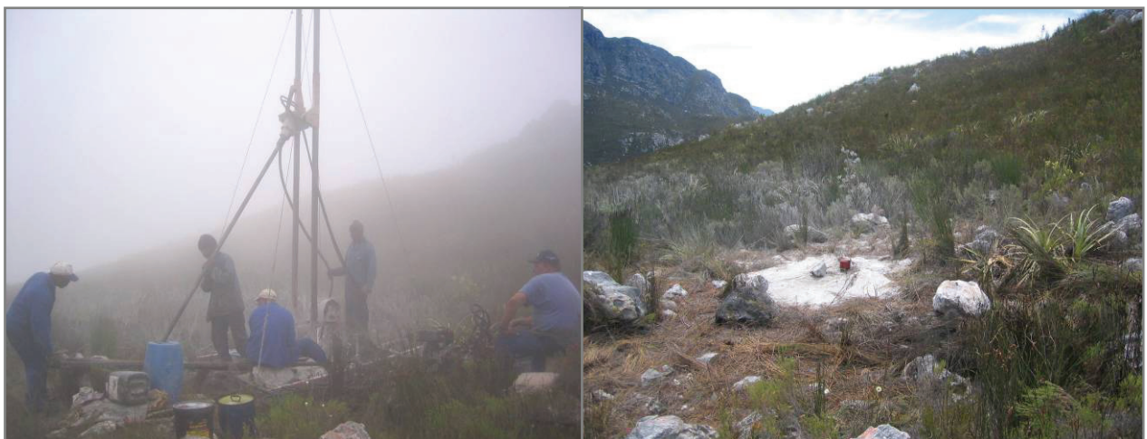
Figure 3-6 The photo on the left shows the KA2 drill site during drilling in misty weather. The photo on the right shows the capped borehole after drilling and the limited footprint of impact from the portable drill rig.
