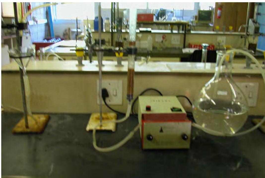
Figure 3.2: Column setup for adsorption and regeneration experiments with seaweed
