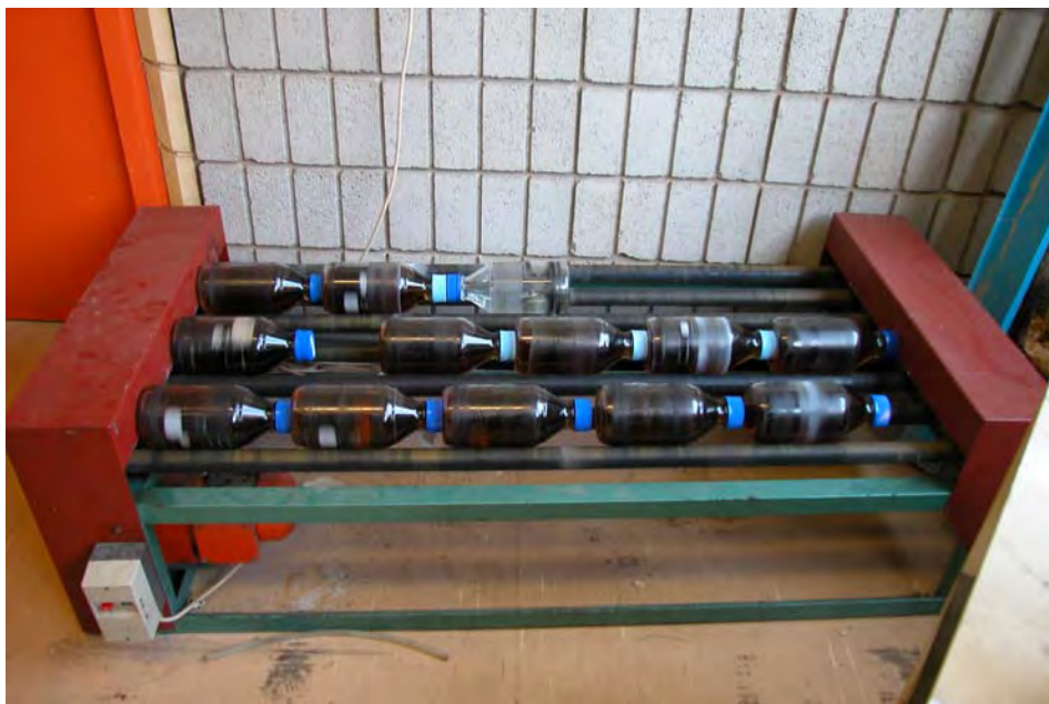
Figure 3.1: Batch adsorption tests taking place in glass bottles on a roller system
