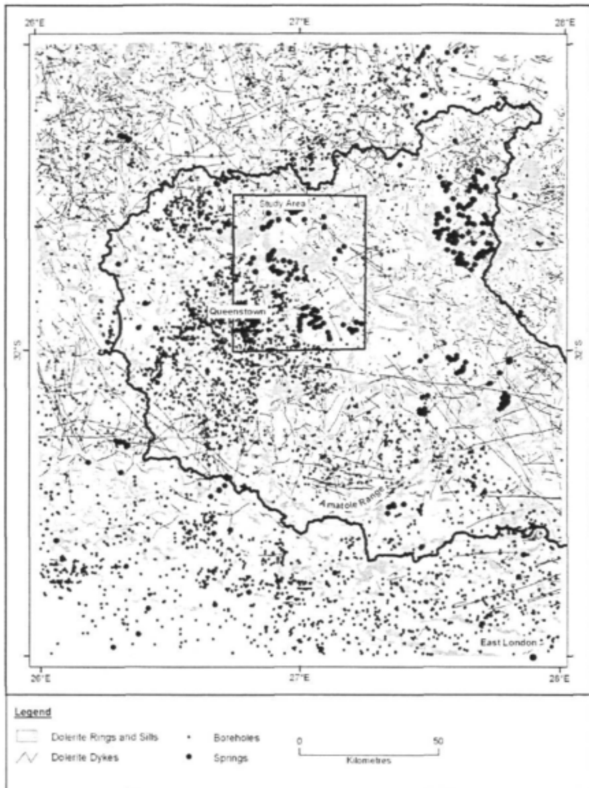
Figure 7: Map of the dolerite dykes, rings and sills of the catchment area also showing the distribution of borehole and spring occurrences.
