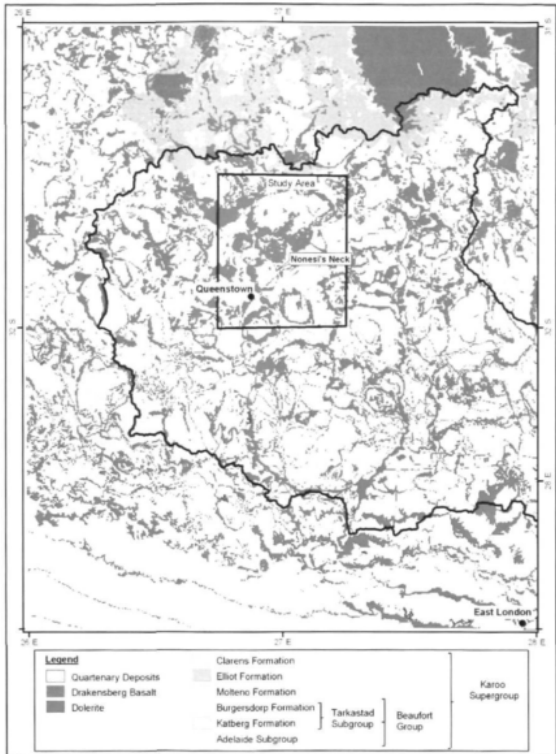
Figure 5: General geology of the Great Kei catchment. Extensive flat dolerite sills are intruded in the Adelaide Subgroup whereas dolerite ring and sill complexes are developed in the Tarkastad Subgroup.
