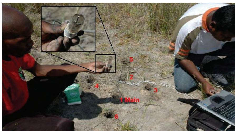
Figure 80: Photograph showing the EC probes and array of monitoring points used to measure flow rate of groundwater in St Lucia (Korsman, 2005)
