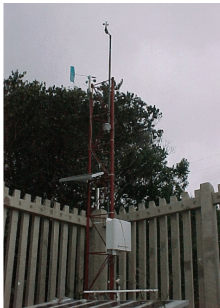
Figure 78: Automatic weather station used for the continuous measurement of rainfall, evaporation parameters and groundwater levels at St. Lucia
