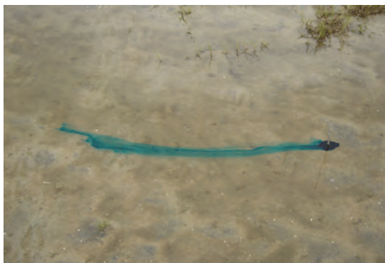
Figure 79: The use of tracers to determine the rate of movement of overland sheet
