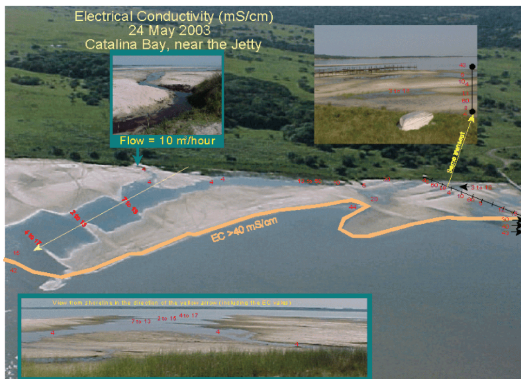
Figure 7.12: Areal photograph of the groundwater seepage at the jetty on the eastern shores of St Lucia on 2003. Concentration contours of Electrical Conductivity are shown from measurements along transects.
