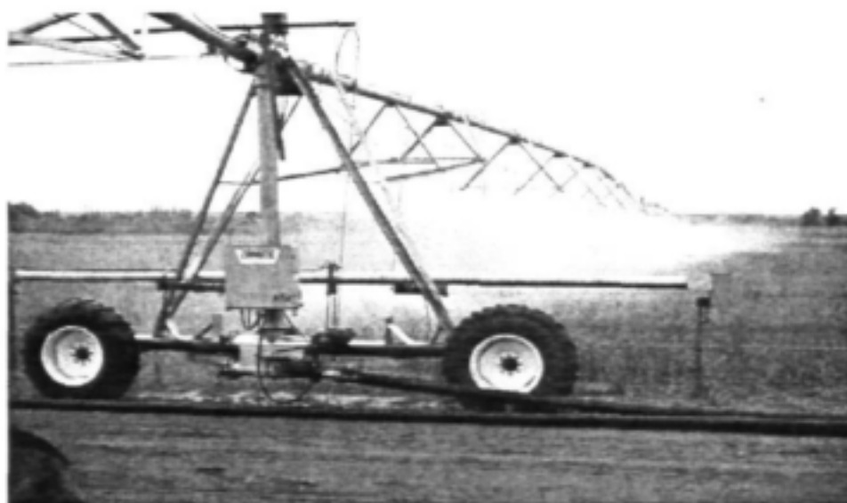
Photo 3.5 A linear irrigation system in operation on the Riet River irrigation scheme (2003)
