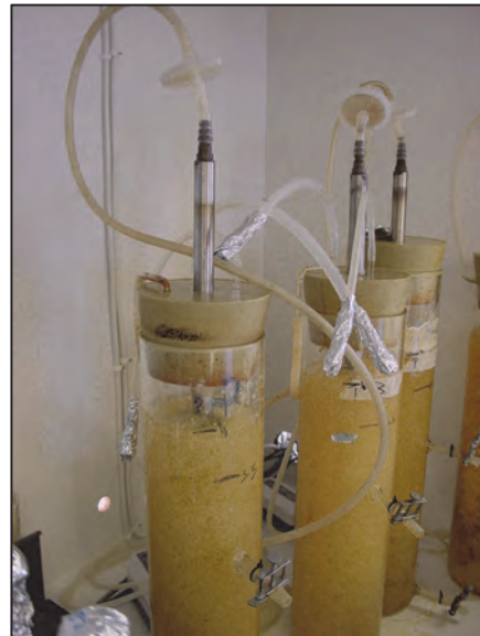
Figure 1.2 Photograph of dense biomass in an airlift bioreactor
