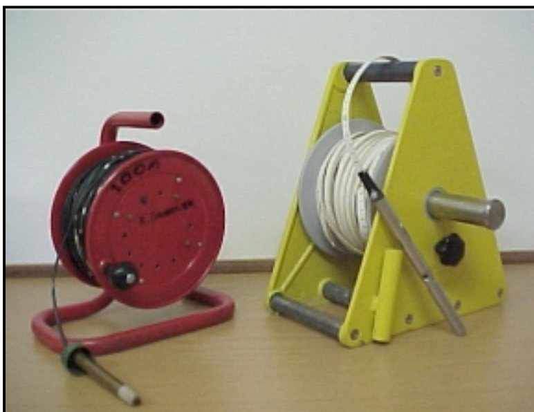
Fig. A7 Two types of dip-meters used for water-level measurement
