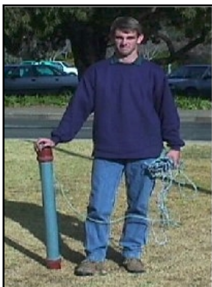
Fig. A5 Slug with known volume to do slug test
