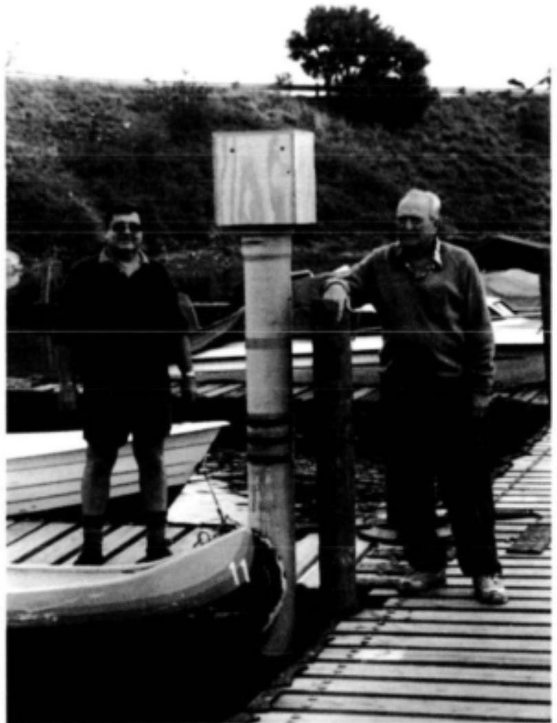
Figure 6.1 The tide gauge on the Bushmans Estuary. The vertical pipe contains the float and counter-weight, while the digital recording system is housed in the box on top. Note that the system must be firmly anchored to avoid any movement, and should preferably be surveyed into datum level. (Photo: E H Schumann)
