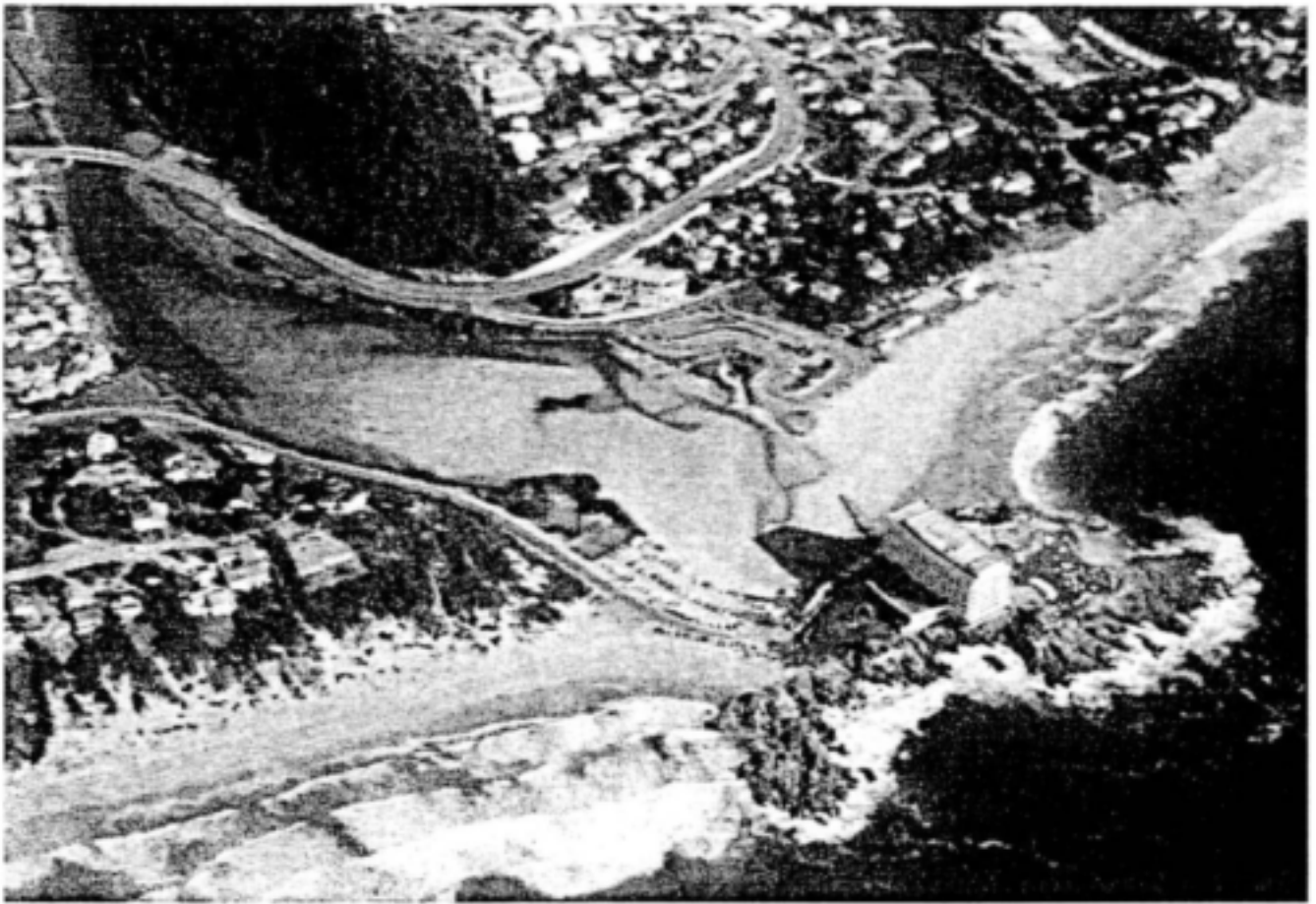
Figure 2.6 The Piesang estuary at Plettenberg Bay during the early 1990's. The flood-tidal delta system composed of marine sand occupies almost the whole lower estuary. Sediment bodies have enlarged since the photograph was taken. Despite the estuary mouth lying sheltered behind a rocky island and being only intermittently tidal, the influx of sand has been very vigorous, possibly the result of a prominent flood dominance of the tide. (Photo: J S V Reddering)
