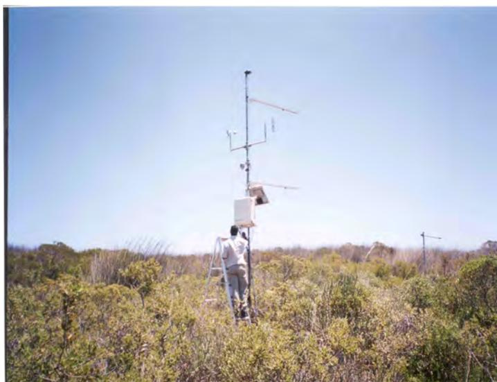
Figure B8: Bowen ratio energy balance system installed at a Rooikrans site (left) and a Strandveld site (right) during summer.
