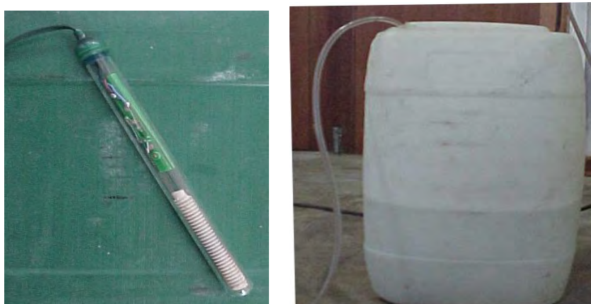
Figure 41. Modified humidifier components: A fish tank heater, left and a 20 litre drum with fish aerator and tubing, right.
