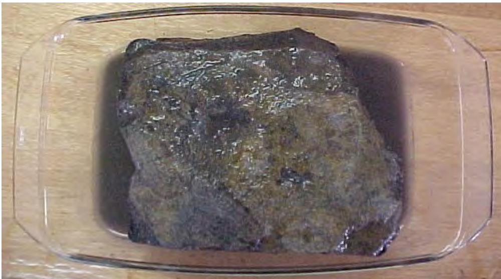
Figure 147. Boulder being treated with hydrogen peroxide at start of test.
