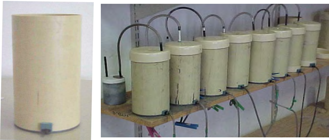
Figure 39. An IGS humidity cell, left and right an array of cells set up at the IGS.
