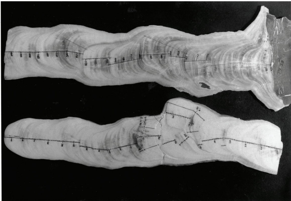
Figure 2.4. Sectioned stalagmite T7 shown in two halves – the basal section is uppermost, and the upper section below. An irregular piece of dolomite is still attached to the base. The slightly altered sampling directions are marked in ink along the growth axes, and small, numbered sample holes. Where complexity was observed in the growth direction, several lines were sampled. Humate staining is clearly visible, particularly in the lower half, and in a limited section of the upper half.
