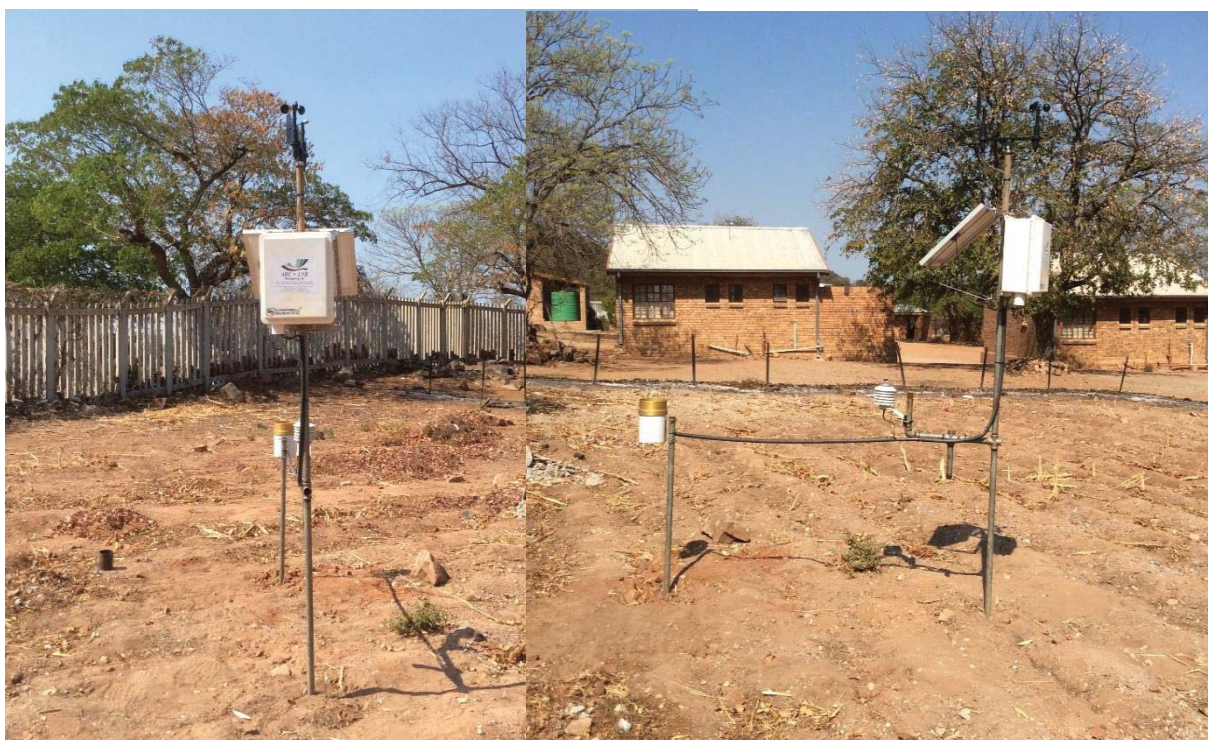
Figure 6: Installed weather station at Sanari
