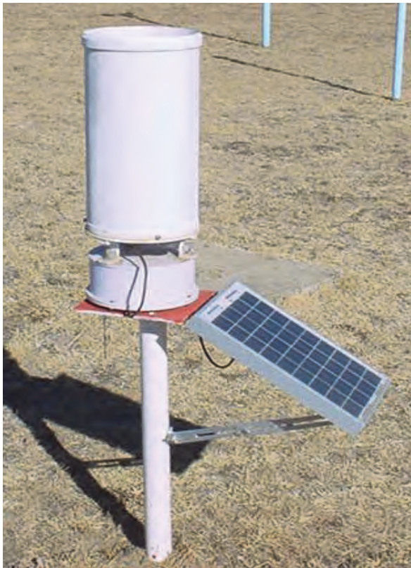
Images of the cell phone modem, electronic component board and the complete rain gauge installation respectively.
