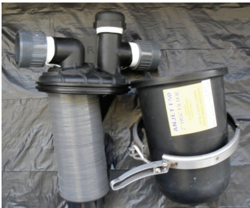
Fig. 5.9 The ANJET F50 disc filter that replaced the sand filter.
