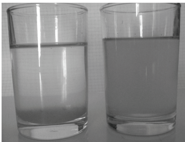
Fig. 3.3 Turbid water from the site. Left: After 5 days standing (~10 FNU). Right: fresh from the tap (~120 FNU).
