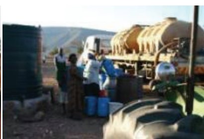
Figure 2.7e: Tanker filling containers, before filling storage tanks (Note the storage tank spigot front left)
