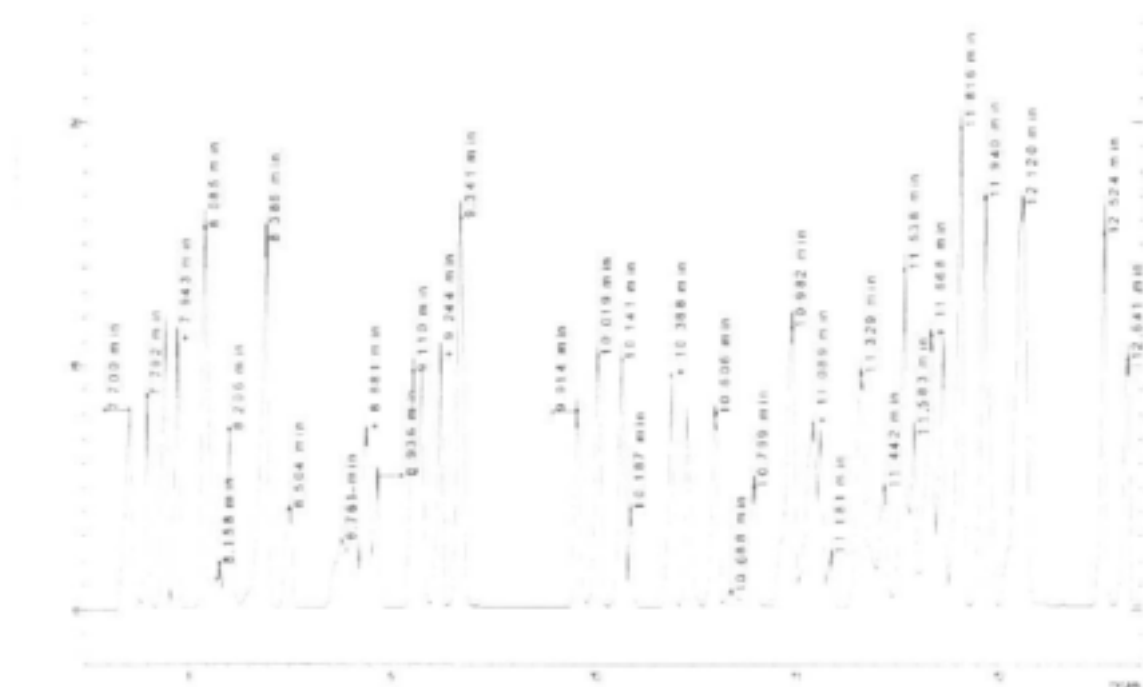
Figure 6.6: Chromatograph showing the peak intensities and retention times of some of the compounds in the standard mixture.
