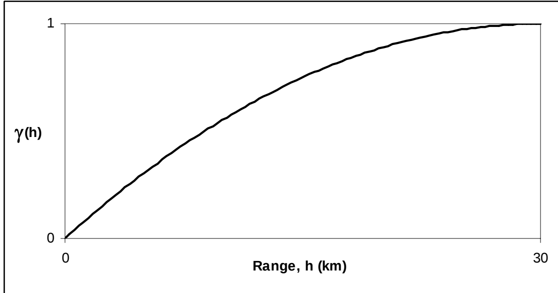
Figure 5.23 Average standardized semivariogram of Radar-rainfall in the Horizontal Plane Relative to a Gauge Position
