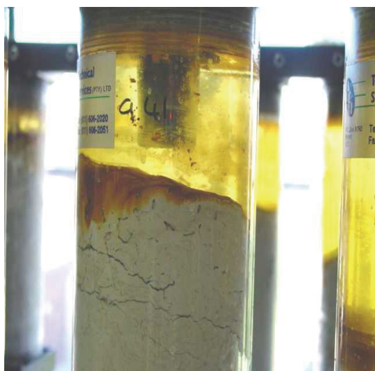
Figure 4.2: Iron deposition on the surface of the ash during column tests.
