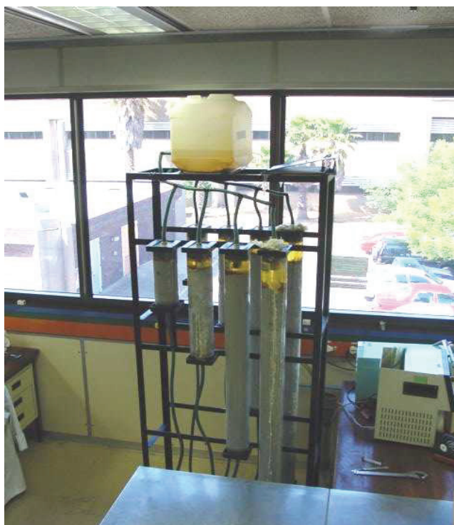
Figure 4.1: Gravity fed AMD through Ash columns
