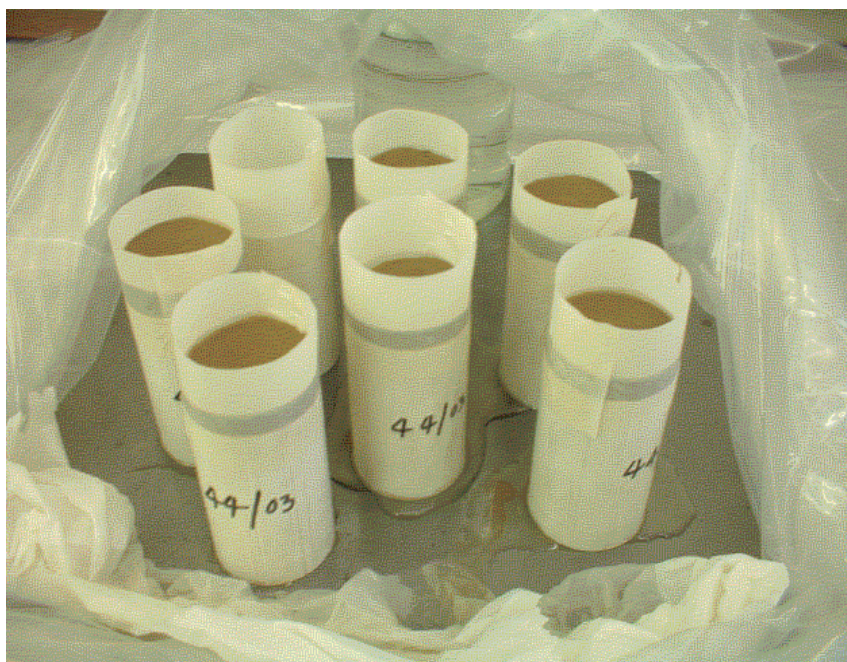
Figure 5.1: Solid residues with binder cured in plastic cylinders for strength development testing at Miningtek laboratory.
