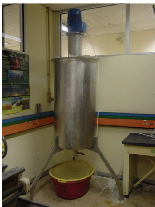
Figure 2.54: Pilot scale mixer with 250 L tank capacity and Turbulator/aeration unit.
