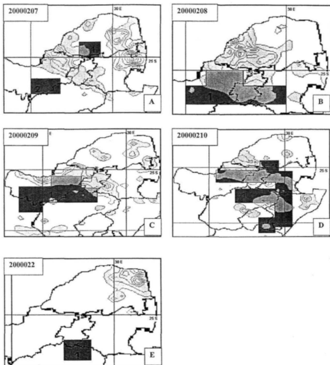
Figure 4.6.2 THERIS results for the Eta data. The blocks indicate the areas where heavy precipitation is predicted. The shaded areas are observed rainfall with the first isohyet at 20 mm. Up to 20 mm rain is possible outside the 20 mm isohyet.
