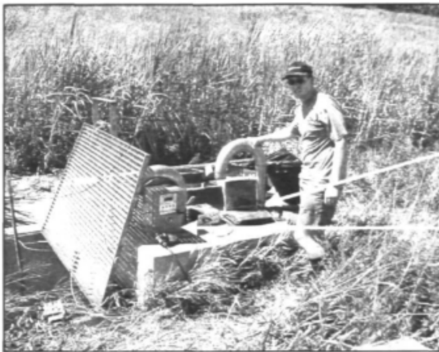
Figure 3.2.6: Air Induction Box used in field setup
