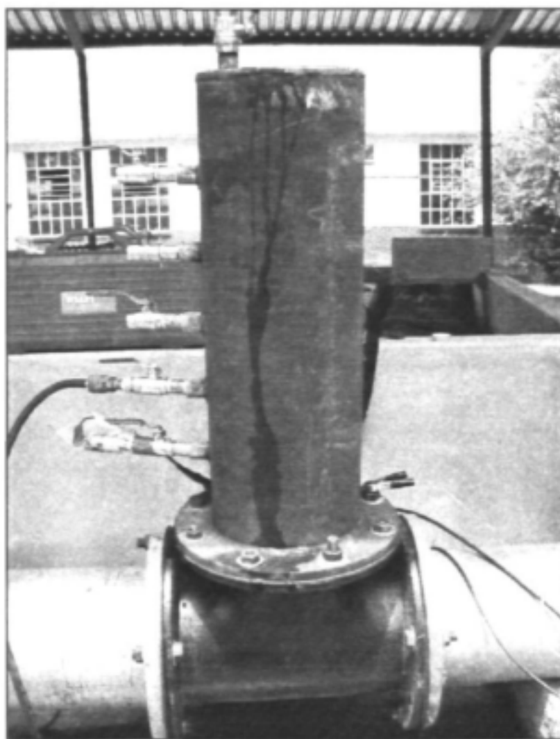
Figure 4.4.11: T-piece for inducing various volumes of air
