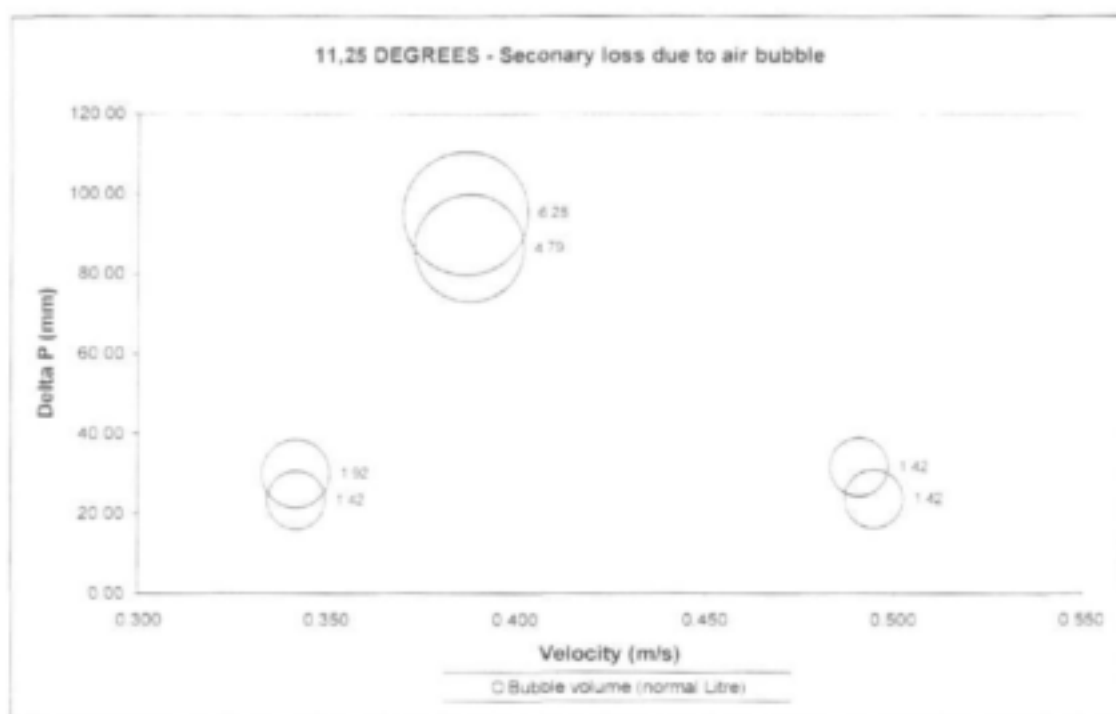
Figure 4.5.8: Graphical presentation of bubble volume measured against secondary energy loss
