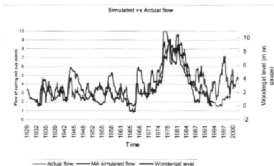
Fig. A. 4. Graph showing the good correspondence between the measured flows of Schoonspruit eye and those simulated by the new recharge formula. Excellent correspondence with the Wondergat levels is shown when the latter is lagged by 5 months.
