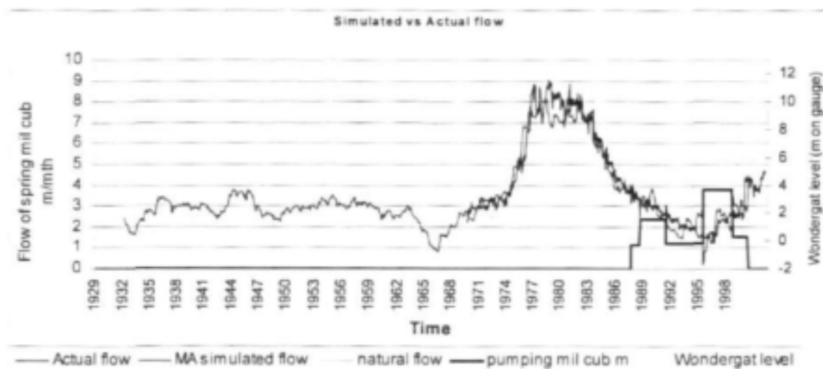
Fig. B.7 The flow of the Schoonspruit eye with pumping which had to be introduced to obtain a good simulation between the measured and simulated groundwater levels
