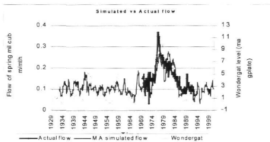
Figure 9: Graph showing the correspondence between the measured flows of Buffelshoek eye and those simulated by the new recharge formula.
