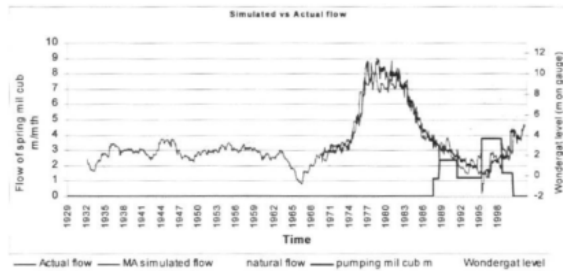
Figure 8: The flow of the Schoonspruit eye with pumping, which had to be introduced to obtain a good simulation between the measured and simulated groundwater levels
