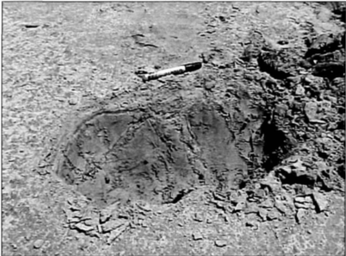
Figure 2.2.1(d): A surface oxidised zone and near-surface preferential pathways visible through iron staining (Bezuidenhout and Vermaak (2002).
