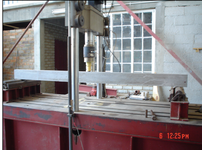
Figure 38: Testing of edge beams
