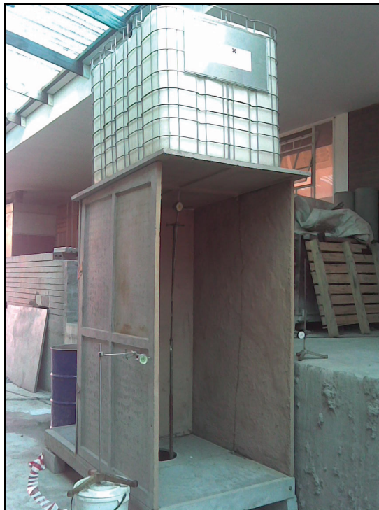
Figure 42: Load on roof of VIP superstructure
