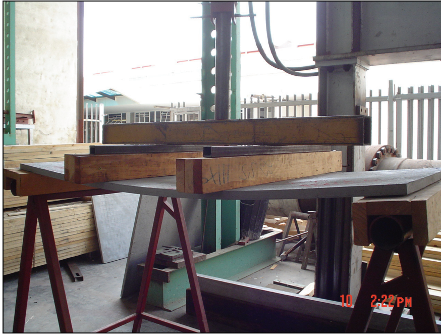
Figure 40: Test setup for wall panels
