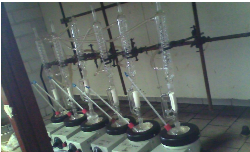
Figure 7: Soxhlet extraction set up with six simultaneous extractions of PAHs from sludge samples
