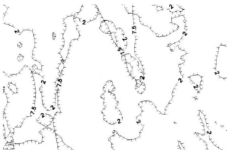
Fig. 41. The 2° slope threshold line (blue) and the EM38-based salinity threshold line (red) for the Glenrosa sub catchment with the direction of hatching showing areas with less salinity (red) and areas with smaller slope (blue)
