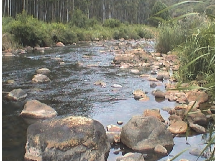
Figure 7.9 View of the Elands River site for a discharge of 0.78\text{m}^3/\text{s} , showing the large roughness elements (Photo A Birkhead)
