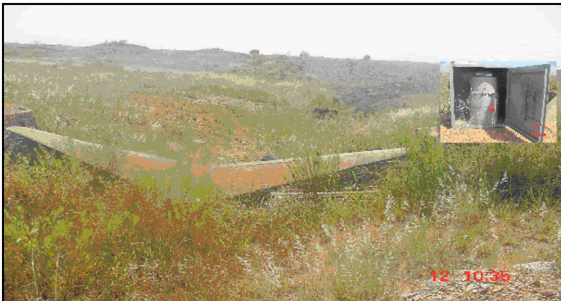
Figure 2.22 Runoff weir at Pivot TWF with a mounted Campbell logger and ISCO water sampler
