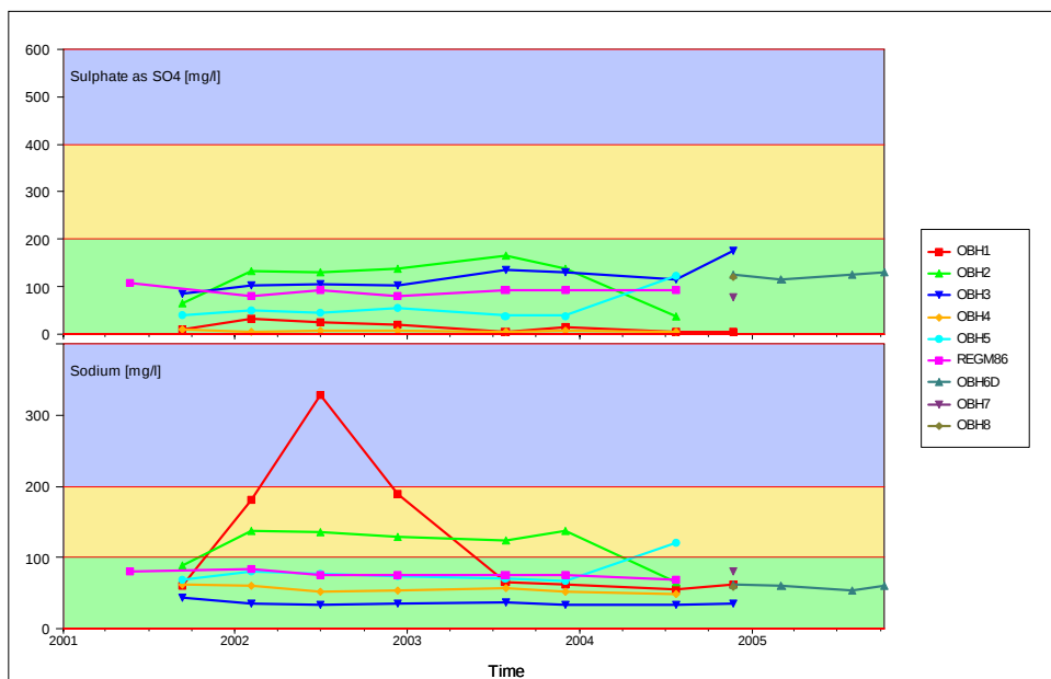
Figure 5.20 Time graphs of sodium and sulphate, the main constituents of the irrigation water.
