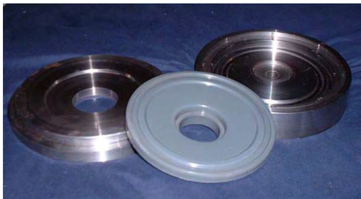
Figure 47: Photograph of the compression mould used to press a manifold flange and the finished PVC product.
