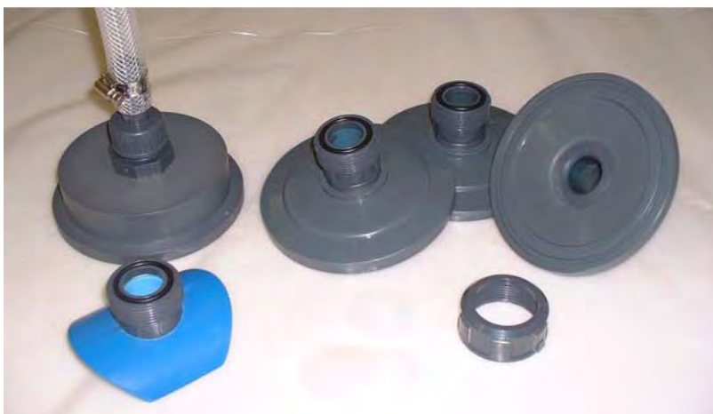
Figure 48: Manifold flanges: a) machined flange with hose-tail connector (left), and b) compression-moulded flange with union stub connector (right).
