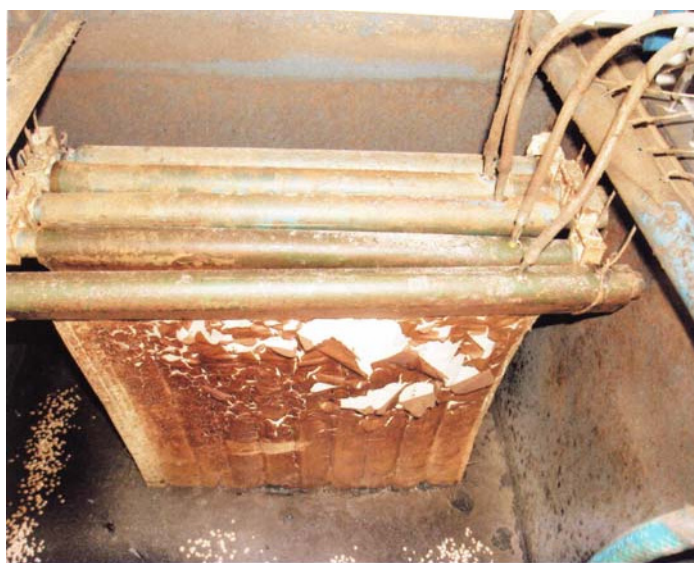
Figure 14: Biofilm peeling from a tubular filter panel, operated in a bioreactor, after the panel has been allowed to dry out completely.
