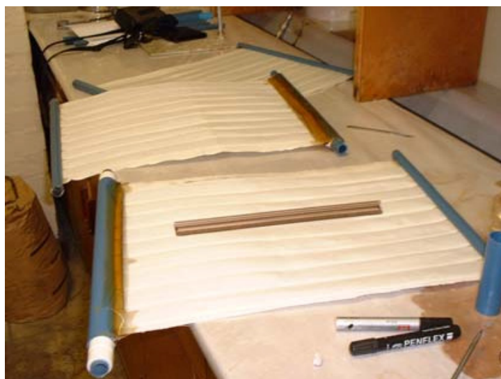
Figure 11:- Tubular woven fabric immersed membrane under construction.
