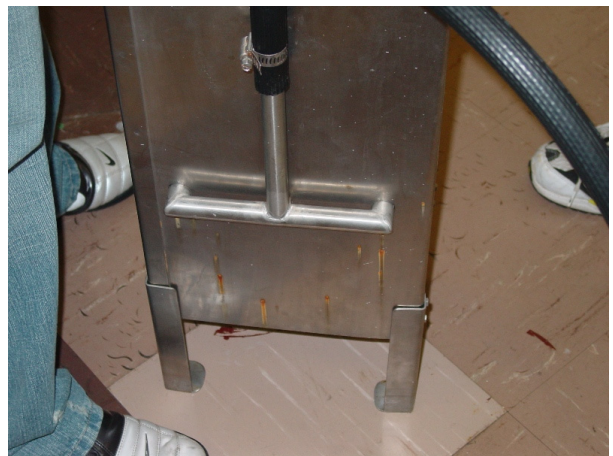
View from side, showing air inlet for gas spargers
