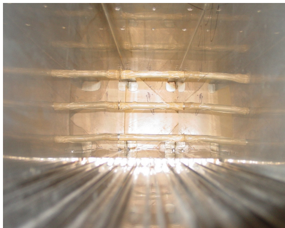
Top view, showing gas spargers
