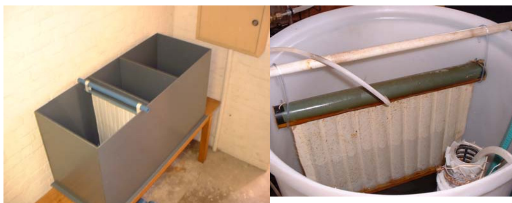
Figure 12:- Bioreactor vessels with one woven tubular fabric membrane envelope.
