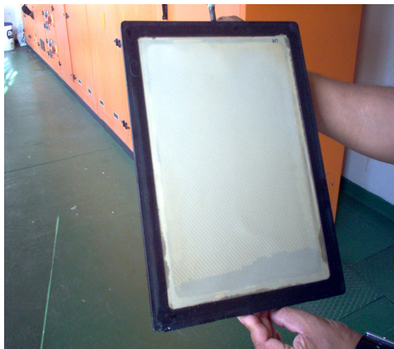
Figure 20: Final module with permeate offtake
