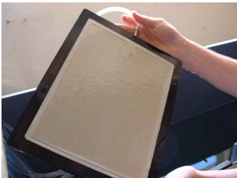
Figure 21: Flat A4 membrane panel after operation on a bentonite feed solution for a number of hours.
