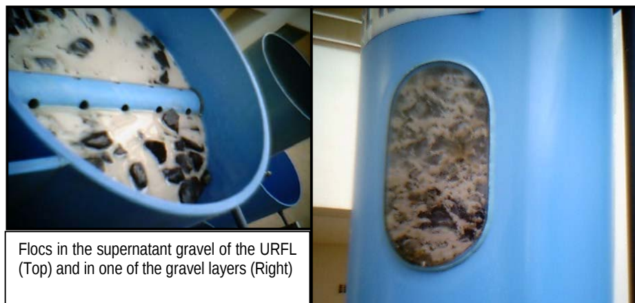
Figure 4-1: Pictures showing floc retention in URFL- 1, PENTECH Plant.
