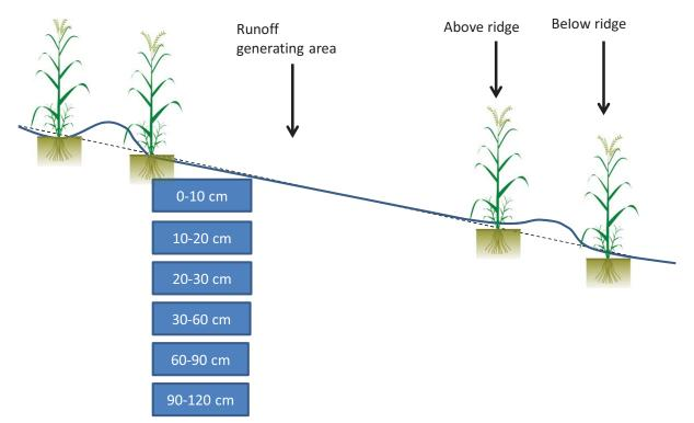
Figure 3.6: Soil sampling procedure for gravimetric moisture content at different positions of a rainwater harvesting setting
