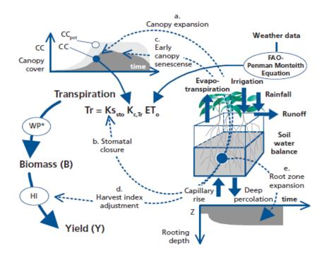
Figure 3.7: Schematic representation of calculations adopted by AquaCrop, with dotted arrows showing the processes affected by water stress. CC is canopy cover, HI is harvest index, WP is water productivity, normalised for ETo and air CO<sub>2</sub> concentration (Adopted from Reas et al., 2009).
