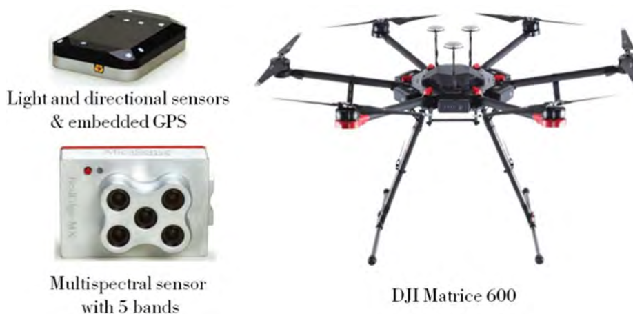
Figure 2. Multi-rotor DJI-Matrice 600 and the MicaSense RedEdge-MX sensor used to capture high-resolution imagery
