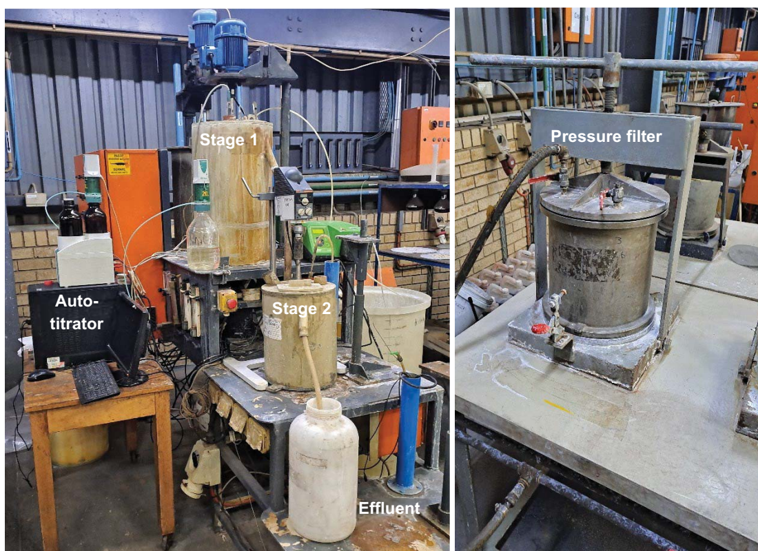
Figure 3-2. Photographs of the pilot-plant setup (left), and the filter press (right)
