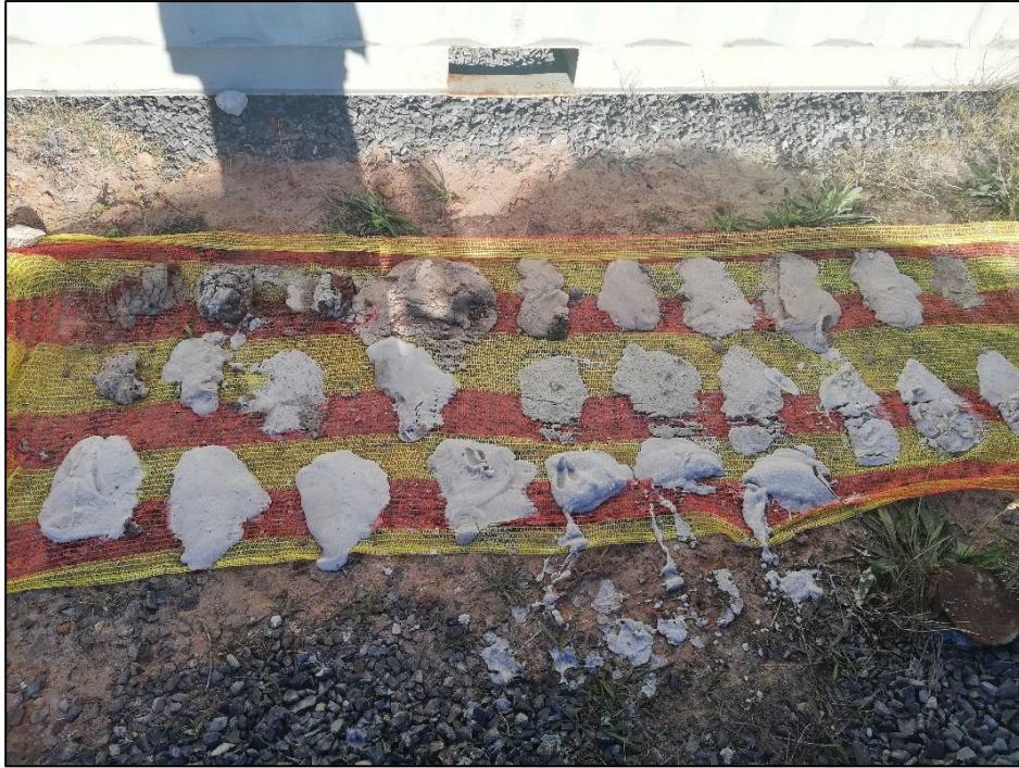
Figure 6. Muddy, indistinguishable drill samples from mud-rotary drilling at the pilot site.
