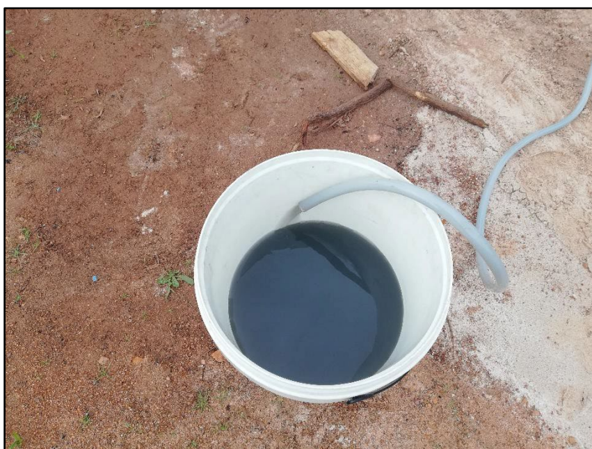
Figure 34. Black water observed during sampling, caused by the drilling of mud residue.
