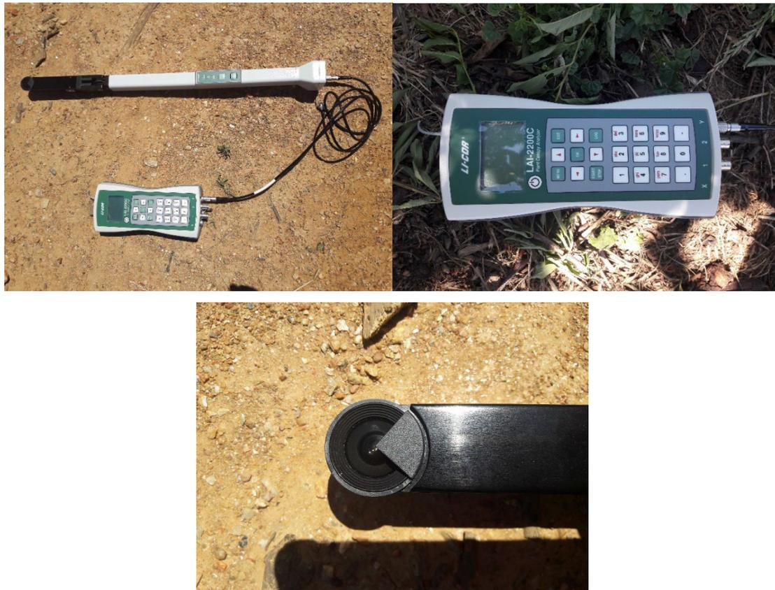
**Figure 4.4** Components of the LAI-2200C plant canopy analyser: console and wand (top left); close-up of the console (control unit); and close-up of the “fish-eye” light sensor installed on the wand.
