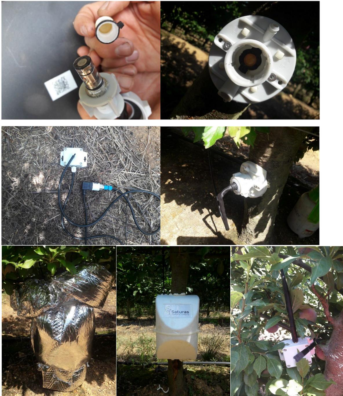
**Figure 4.5** From top left clockwise: Saturas sensor for measurement of stem water potential; Sensor mounting: a hole in the tree trunk is drilled until the appearance of soft tissue; Sensor installed in the trunk; Antenna relay that transmits the sensor's signal to a receiver; Saturas sensor installed in a plum tree trunk and covered with polystyrene; Reflective cover for isolation; and Pressure transducer installed to keep track of irrigation timing.
