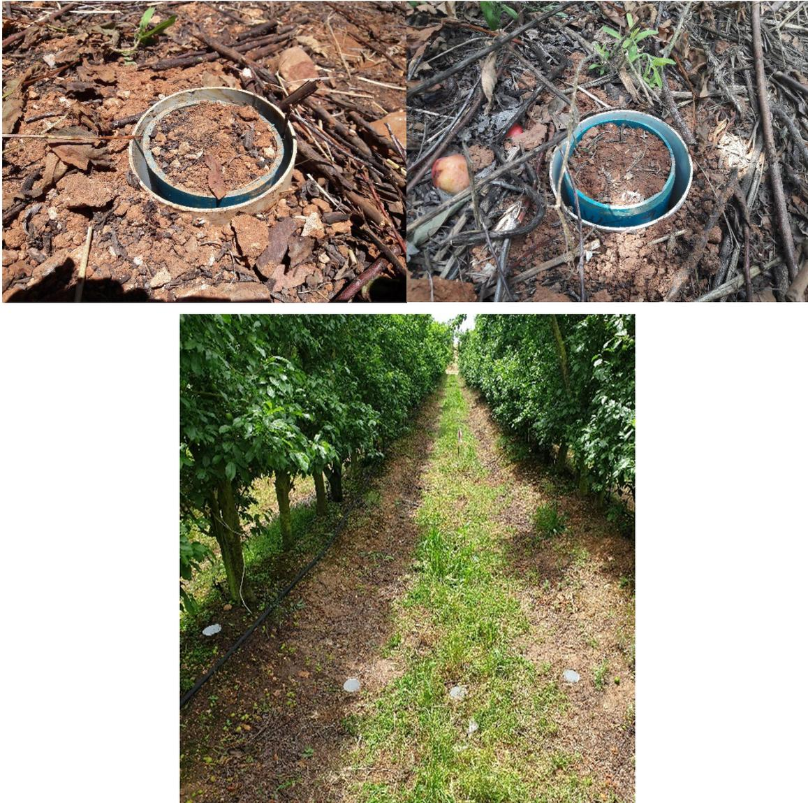
**Figure 4.3** Top: In-house manufactured micro-lysimeters installed in the field for measurement of soil evaporation. Bottom: Micro-lysimeters installed across the tree rows.
