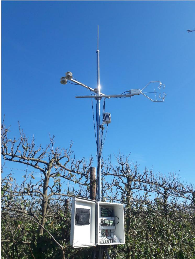
**Figure 4.10** The eddy covariance flux tower mounted in an African Delight orchard at Klipboschlaagte farm.
