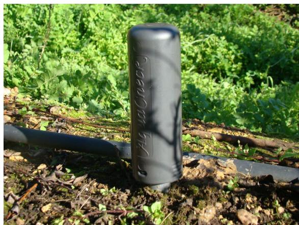
**Figure 4.1** a) AquaCheck probe (top left), b) hand-held wireless AquaCheck Basic II data logger (top right), c) installation of AquaCheck probes with a portable motor drill (bottom left) and d) installed AquaCheck probe (bottom right).
