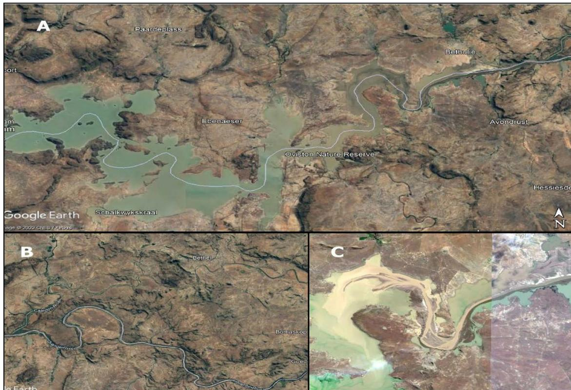
**Figure 6.10:** Sedimentation in the Gariep dam
