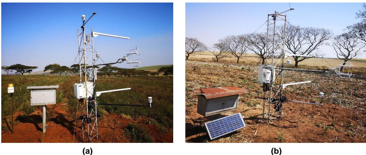
**Figure 4-3** Micrometeorological equipment installed at the (a) taro and (b) OFSP trial sites located within the Fountainhill Eco-estate
