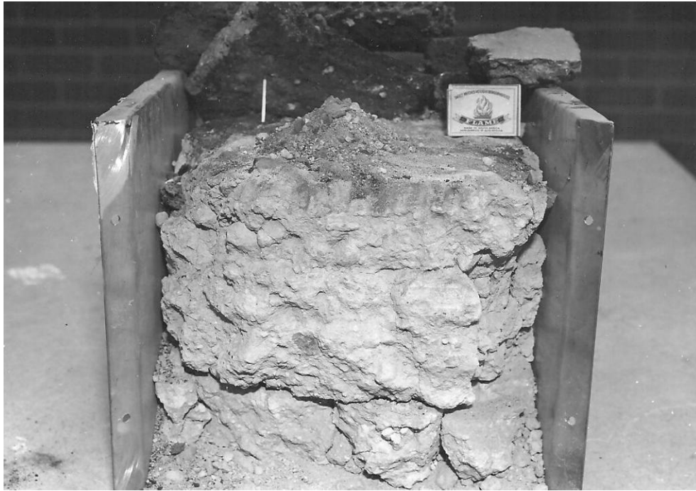
Figure A.7.1. Loose interlayer between asphalt and lime stabilised calcrete base course on intact, undisturbed sample of base and subbase from Oshivello-Oshakati road
