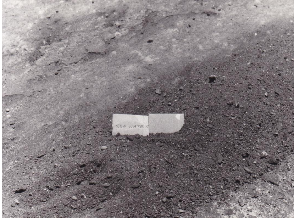
Figure A.4.2. After brooming some of the flaking prime on the seawater calcrete base
