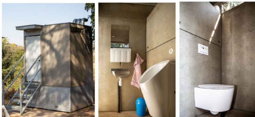
Figure 20: Images of the Blue Diversion Autarky Toilet (BDAT) prototype, tested in eThekweni, South Africa (taken from Sutherland et al. (2021a))
