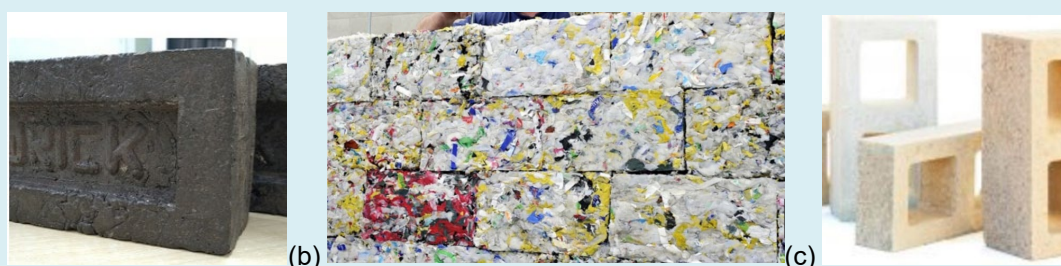
Figure 8: The Angirus Ind Pvt. Ltd., Wricks brick innovation, (b) the Replast blocks (taken from EngineeringforChange (2022)).
